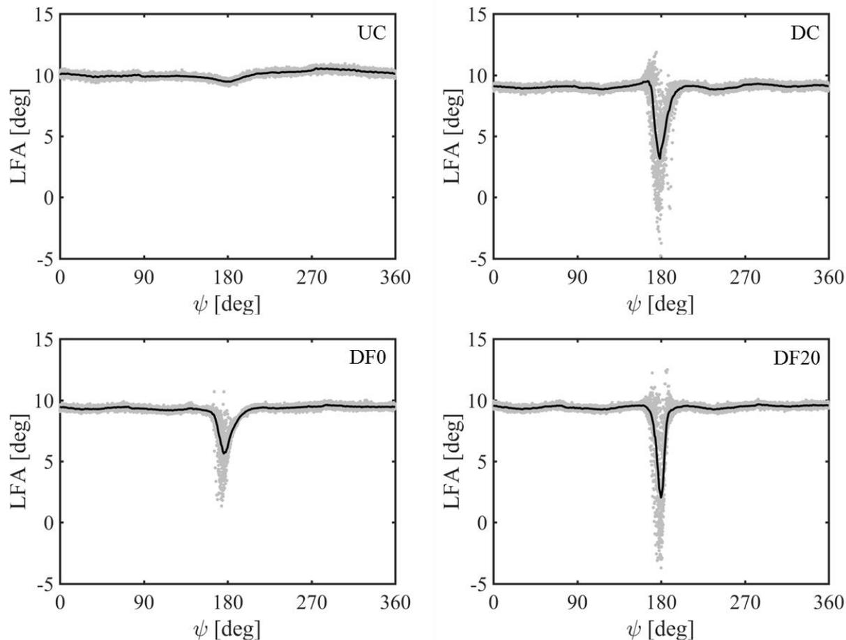
**Fig. 4 Local flow angle as function of azimuthal angle at  $r/R=0.67$  and  $U_\infty=7\text{m/s}$ . The grey dots indicate instantaneous measured values while the solid black line indicates the cycle-averaged measurements (averaging all values for a given  $\psi$ ).**
