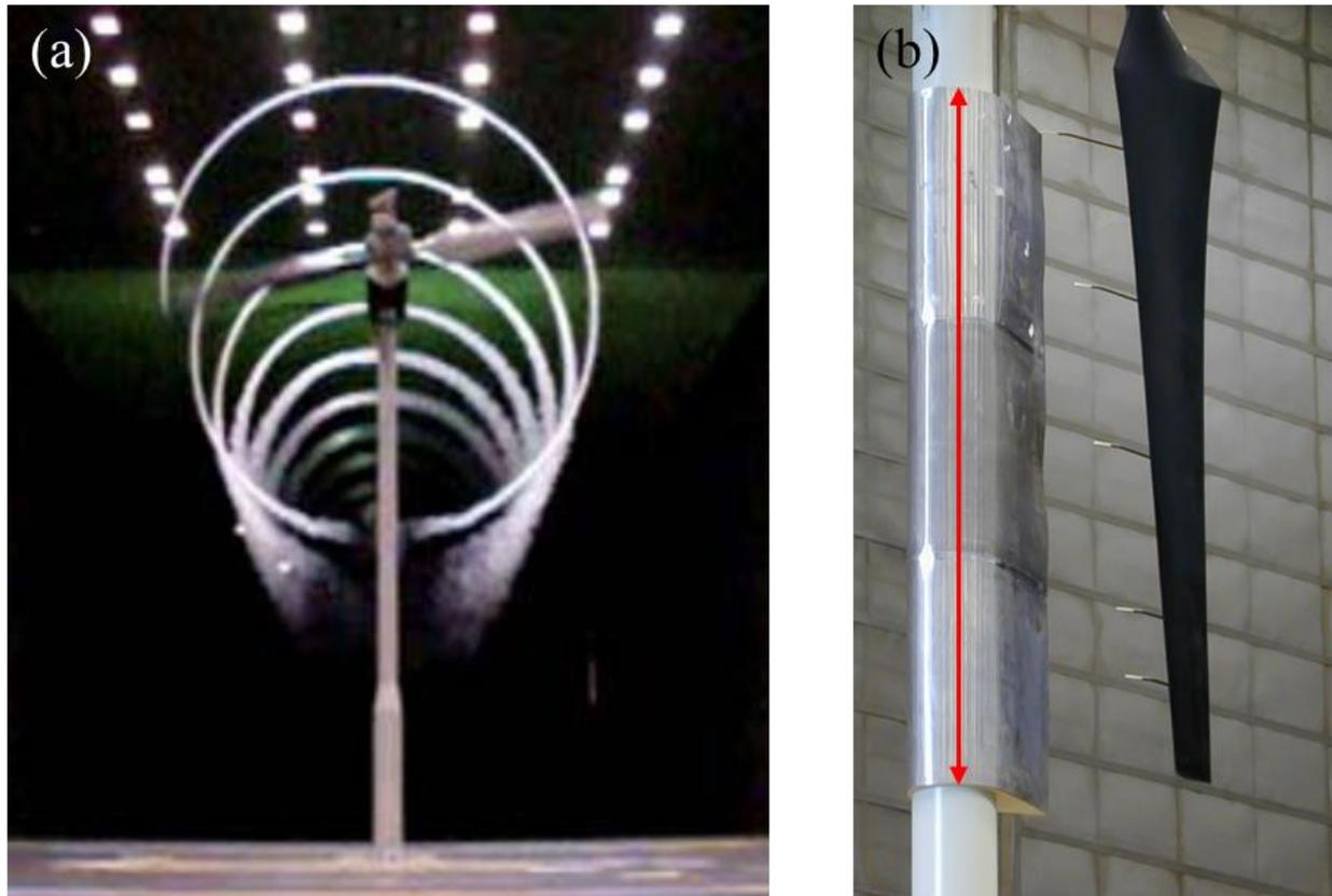
**Fig. 1 UAE experimental configuration in the NASA Ames tunnel: (a) flow visualization of tip vortices, and (b) UAE tower fairing (with arrow indicating vertical extent) upstream of a UAE blade instrumented with 5-hole pressure probes**
