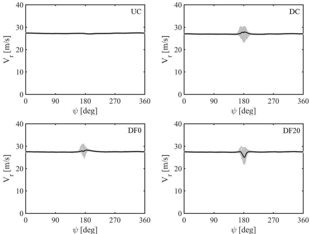
**Fig. 5** Resultant velocity as function of azimuthal angle at  $r/R=0.67$  and  $U_\infty=7\text{m/s}$  using same symbol representation as in Fig. 4.
