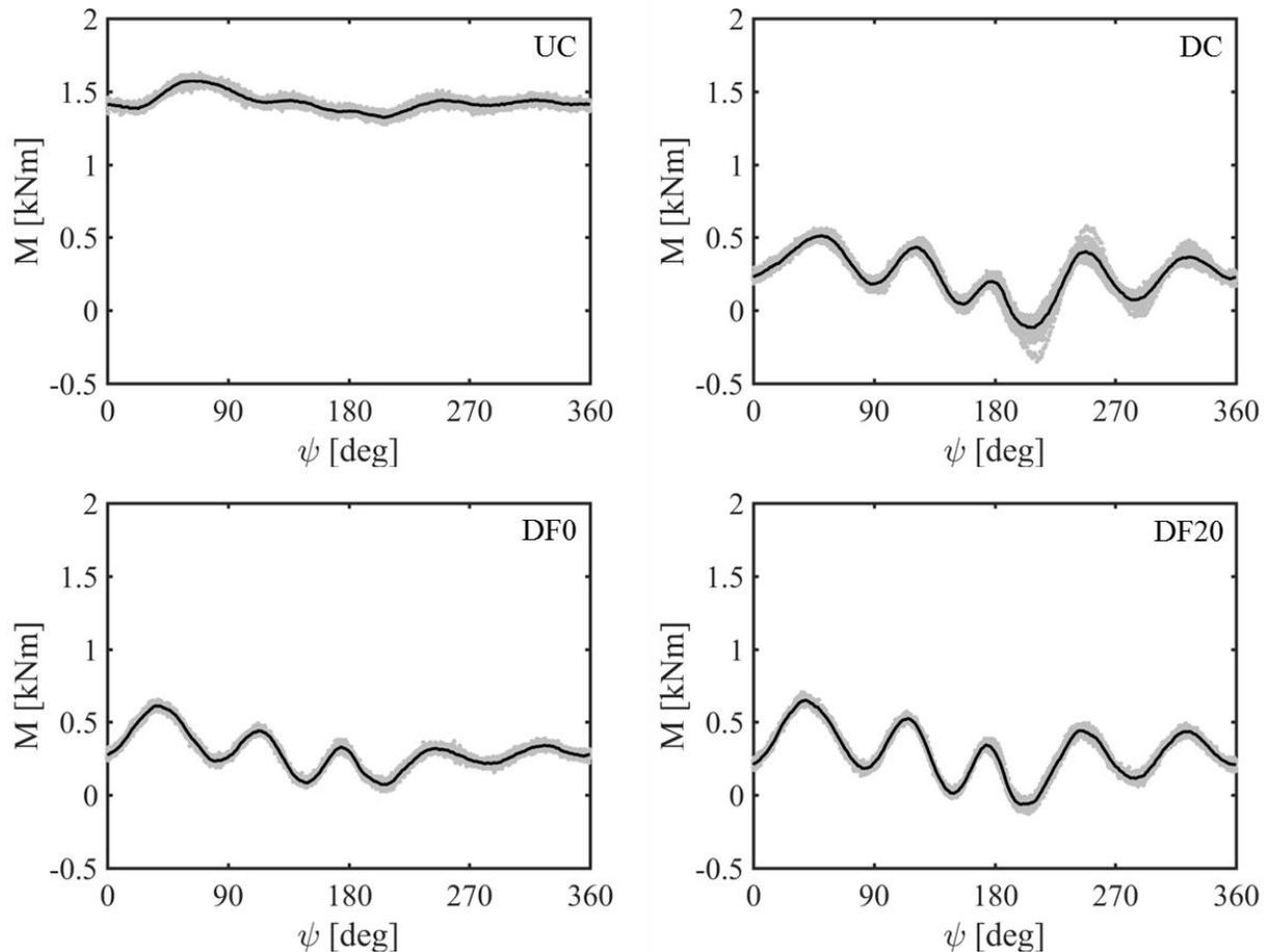
**Fig. 7 Root flap bending moment as function of azimuthal angle at  $U_\infty = 7$  m/s using same symbol representation as in Fig. 4.**
