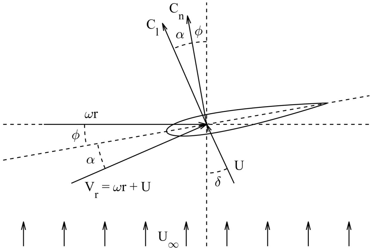
**Fig. 3 Schematic of flow parameters: pitch plus local twist ( $\phi$ ), instantaneous wind deflection ( $\delta$ ), instantaneous wind ( $U$ ), free stream wind ( $U_\infty$ ), angle of attack ( $\alpha$ ), rotational velocity ( $\omega r$ ), where  $C_n$  is normal to chord line &  $C_l$  is normal to the resultant flow ( $V_r$ ).**
