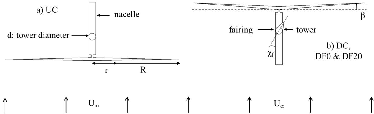
**Fig. 2 Top view turbine schematic: (a) upwind rotor and (b) downwind rotor with fairing free to rotate about tower**
