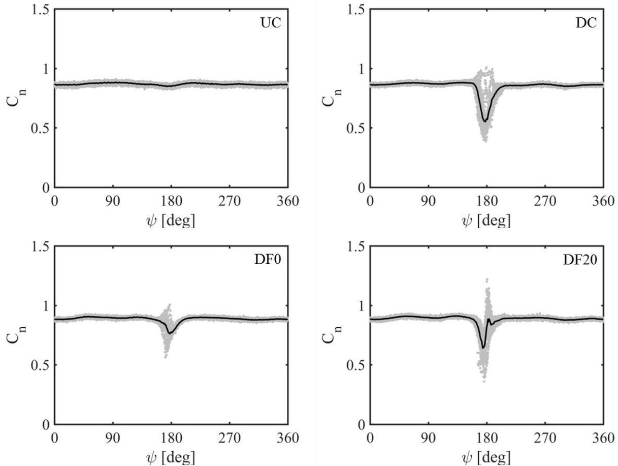
**Fig. 6** Normal force coefficient as function of azimuthal angle at  $r/R=0.63$  and  $U_\infty=7$  m/s using same symbol representation as in Fig. 4.
