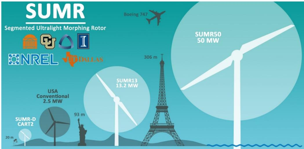
Figure 1: SUMR – Segmented Ultralight Morphing Rotor Concept for Extreme-scale Wind Turbines
