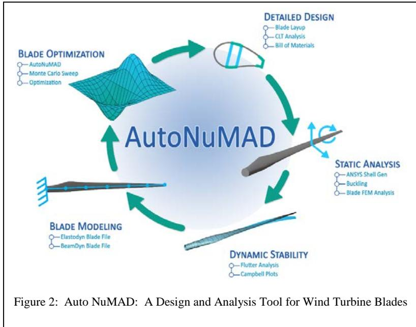
Figure 2: Auto NuMAD: A Design and Analysis Tool for Wind Turbine Blades
